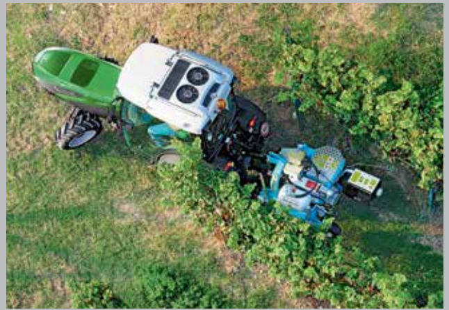
Improved turning radius thanks to a slimmer front support.
