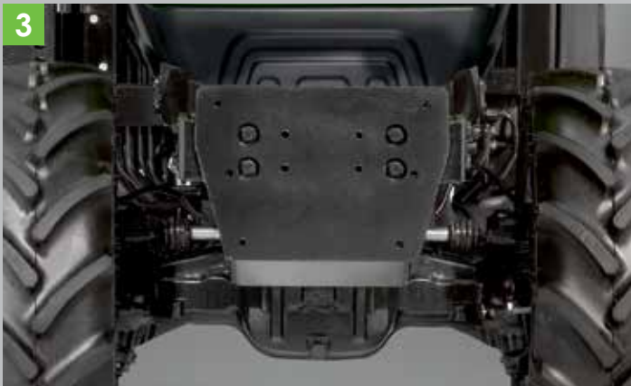
3 Front mounting plate for the fast, secure attachment of special equipment.
