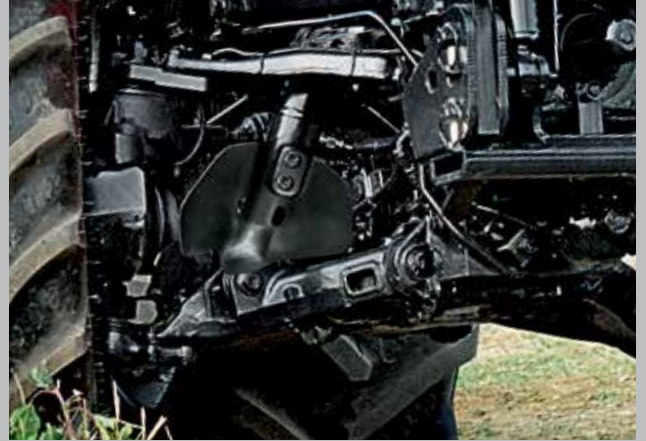
Independent wheel suspension with double wishbone design.
