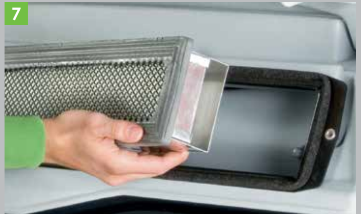
7 The cab air filter prevents dust and chemicals. Clean air inside the cab at all times.
