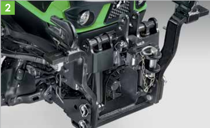
2 Front hydraulics and front PTO for efficient equipment combinations.
