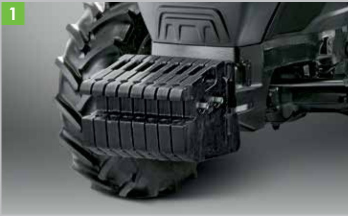
1 Different front weights for working with heavy rear attachments.
