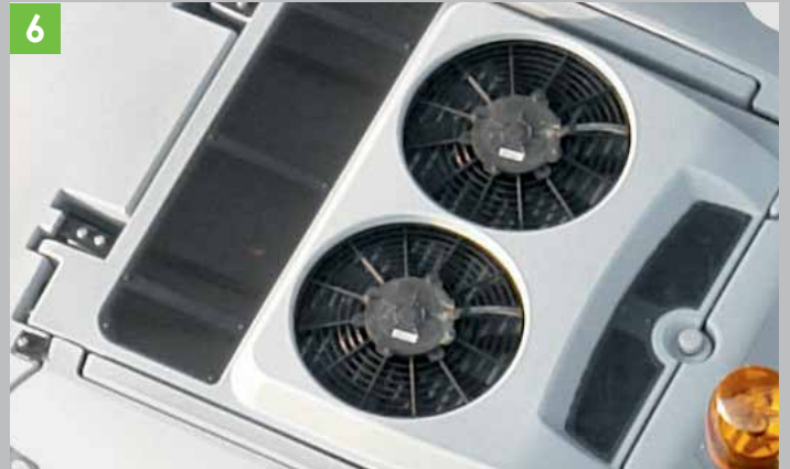
6 High-performance air conditioning system for a consistently pleasant cab working environment.
