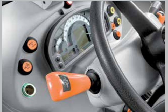
Powershuttle. Change the direction of travel with a single touch.
