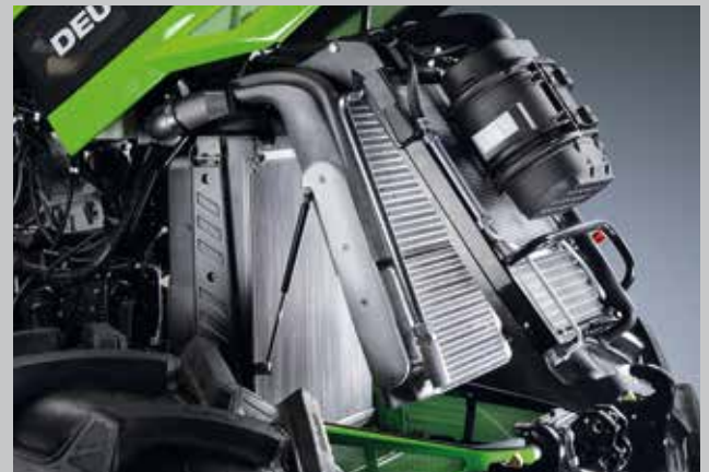
Newly designed cooling system. Fully openable for easy maintenance.
