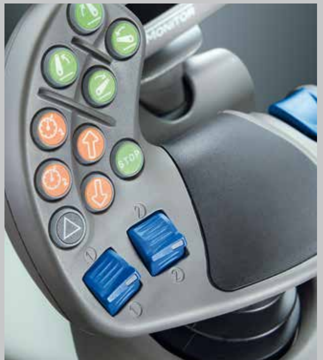
Up to 4 cruise speeds can be memorised to optimise application and efficiency.
