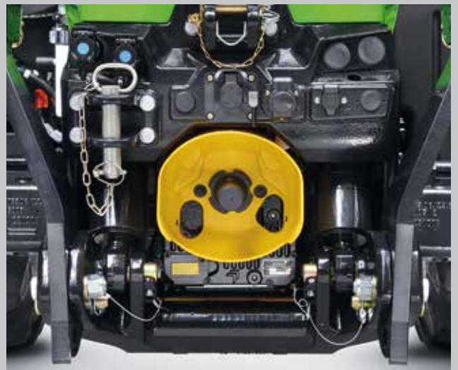
Up to 7 proportional spool valves at the rear and 2 in the front. Front lift integrated to the tractor and closer coupled
