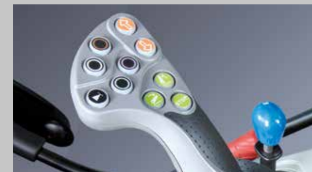
The TTV models are operated using the new PowerCom S joystick. Four buttons can be assigned to any function.
