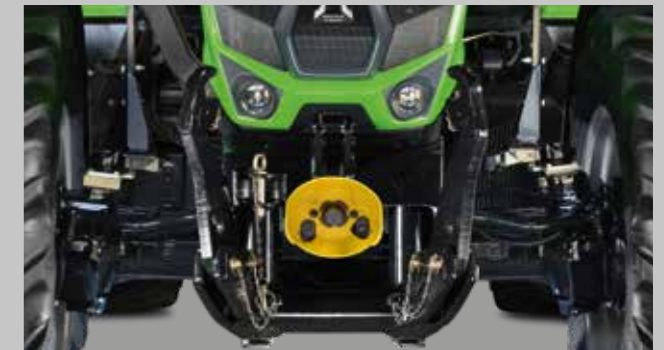
The powerful front linkage can lift up to 2,880 kg. Also available: the ComfortPack with an additional control valve at the front.
