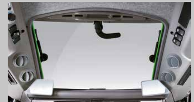
A choice of four roof designs: a transparent sunroof with or without FOPS and an opaque roof with or without FOPS.
