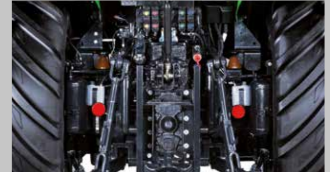
Impressive characteristics: a lifting capacity of up to 7,000 kg, Category III, electronically controlled trailer coupling as standard.
