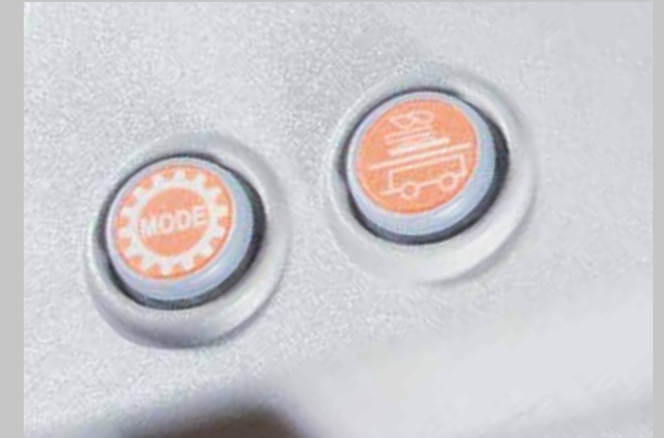
Working mode (FIELD/TRANSPORT) can be selected electro-hydraulically: FIELD/TRANSPORT mode can be changed in standstill or while driving (max. 15 km/h)
