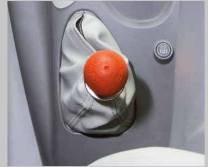
Hydraulic parking brake. A secure position wherever you park your new 6 Series tractor.
