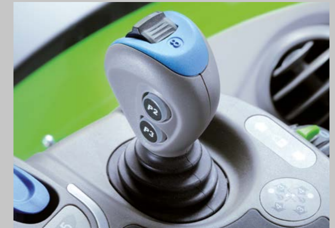
Three hydraulic valves are controlled via a simple joystick with integrated smart wheel.
