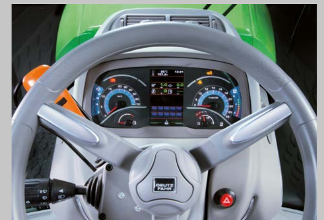
The new InfoCentre provides an overview of operating conditions – in both digital and analogue mode.
