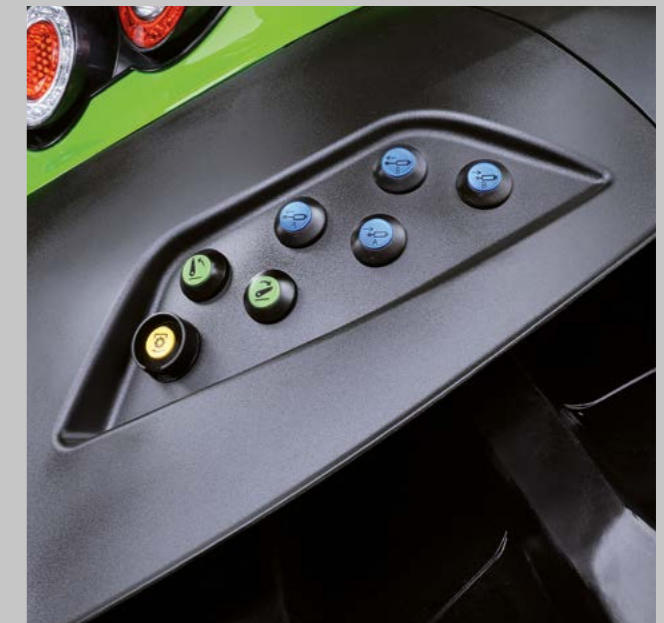
External control of hydraulics and PTO functions from both sides.
