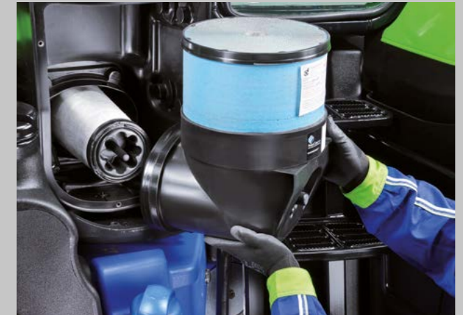
No tools are required for replacing the engine air filter.
