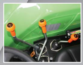
All transmission controls located in the right hand console, complete with mechanical Forward/Reverse shuttle.
