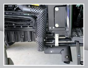
Down swept exhaust combined with foldable ROPS frame gives the tractor exceptionally low clearance.
