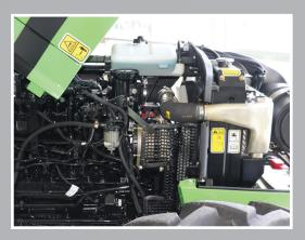
Powerful 4 cylinder engine with maximum output of 75hp.
