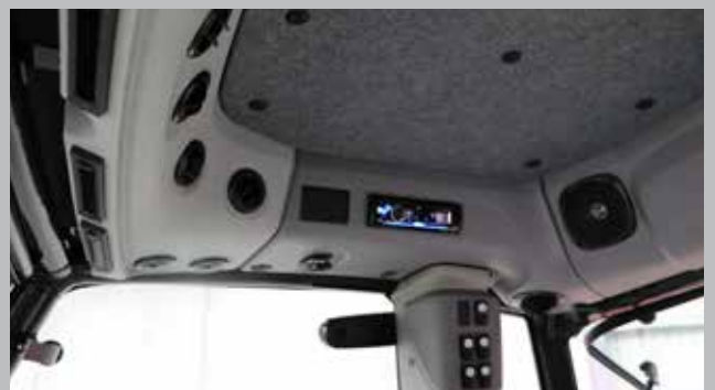
Air vents located throughout cabin.
