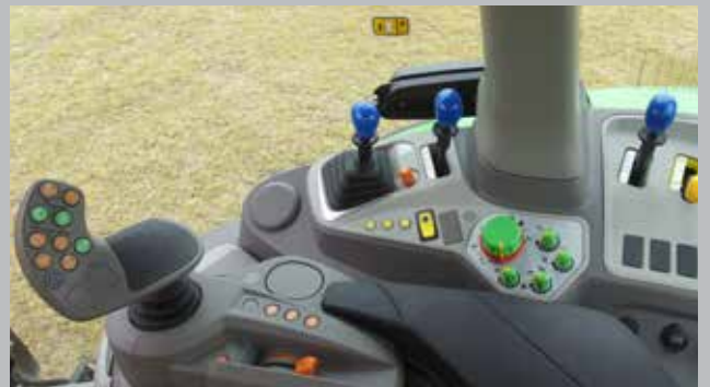
Armrest controls - Summit specification (RC Transmission available for 6185G and 6205G only)
