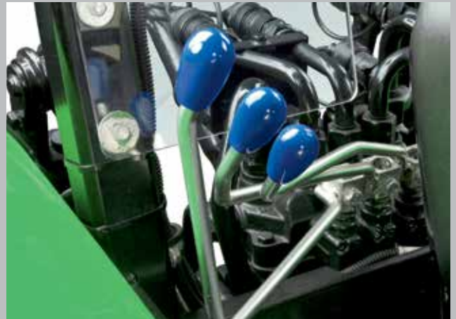
Equipped with up to 3 mechanical auxiliary valves.
