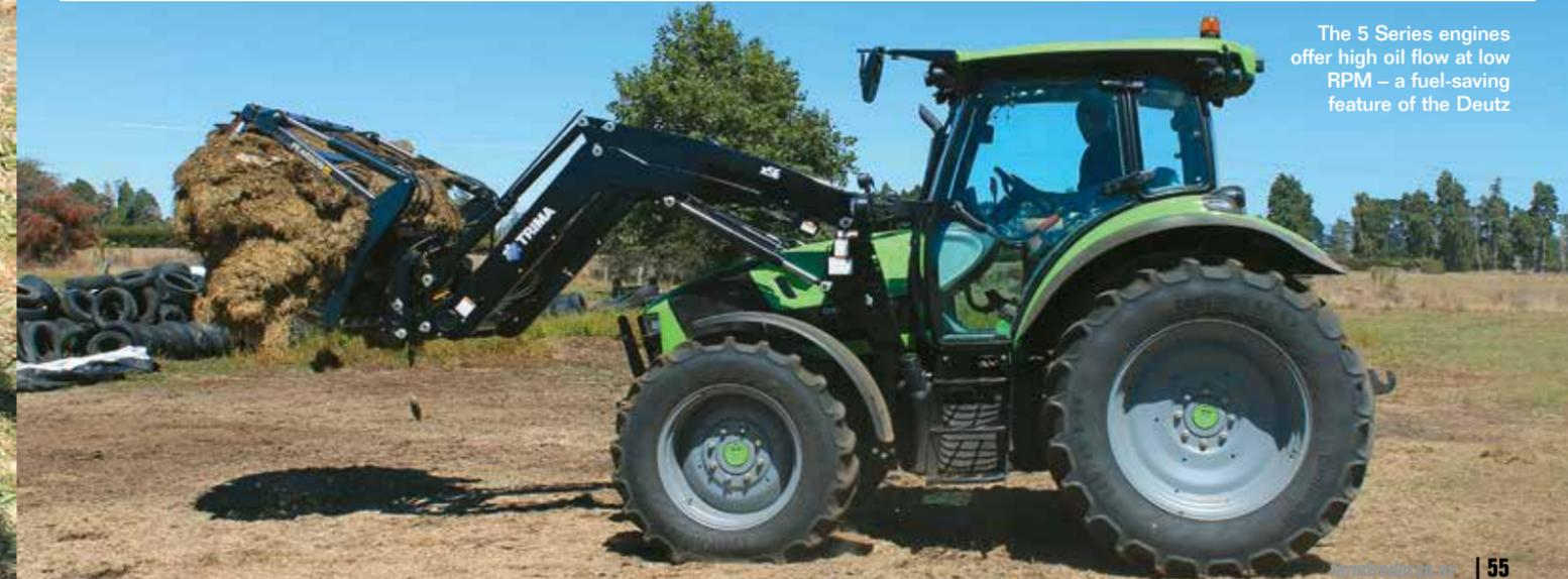
The 5 Series engines offer high oil flow at low RPM – a fuel-saving feature of the Deutz
