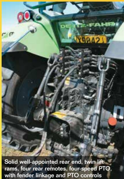
Solid well-appointed rear end, twin lift rams, four rear remotes, four-speed PTO, with fender linkage and PTO controls
