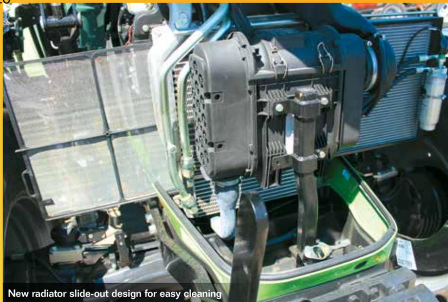
New radiator slide-out design for easy cleaning
