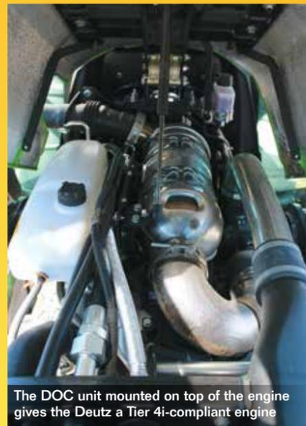
The DOC unit mounted on top of the engine gives the Deutz a Tier 4i-compliant engine
