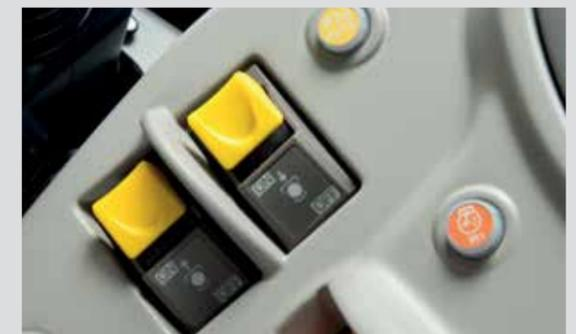
Electro-hydraulic switches to engage PTO.
