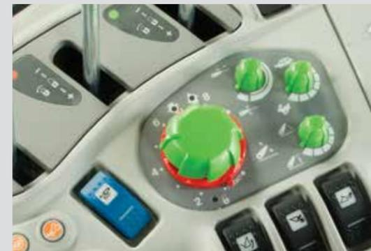
Console with electronic hitch control
