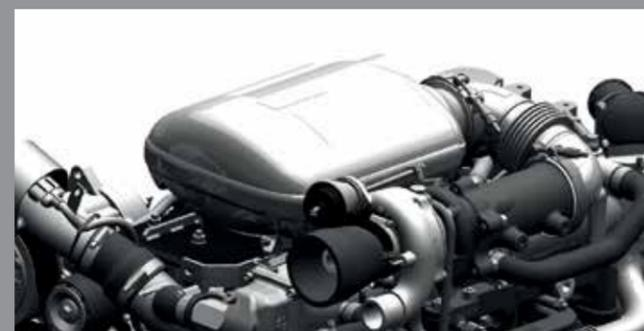
**DOC - (Diesel Oxidation Catalyst):** The exhaust gas oxidation catalyst (DOC) helps reduce pollutants via a "catalytic sponge". It converts the unburned hydrocarbons (HC), the nitrogen oxides (NO) and the carbon monoxide (CO) into carbon dioxide, nitrogen and water in the form of water vapour. Unlike diesel particulate filters (DPF), the DOC remains effective throughout the service life of the engine without any need for regular maintenance or active regeneration.
